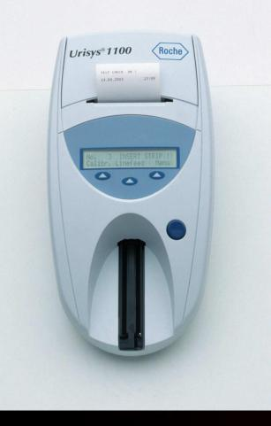
Portable analyzer for small laboratories.
