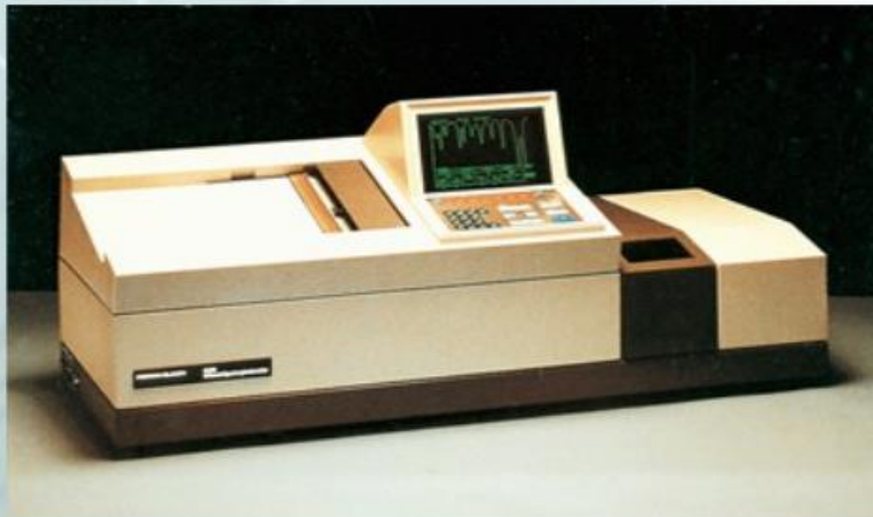
An infra-red spectrometer
