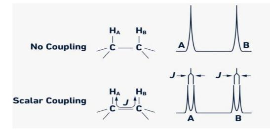
NMR signals from HA and HB emerge as simple peaks when there is no scalar coupling (top). The signals will divide if the two neighboring protons HA and HB exhibit scalar coupling with a constant J (bottom). Because both protons HA and HB are associated with one proton bound to a contiguous carbon nucleus, each proton signal will split into two signals, generating a doublet, with the split distance equal to the coupling constant, J.
