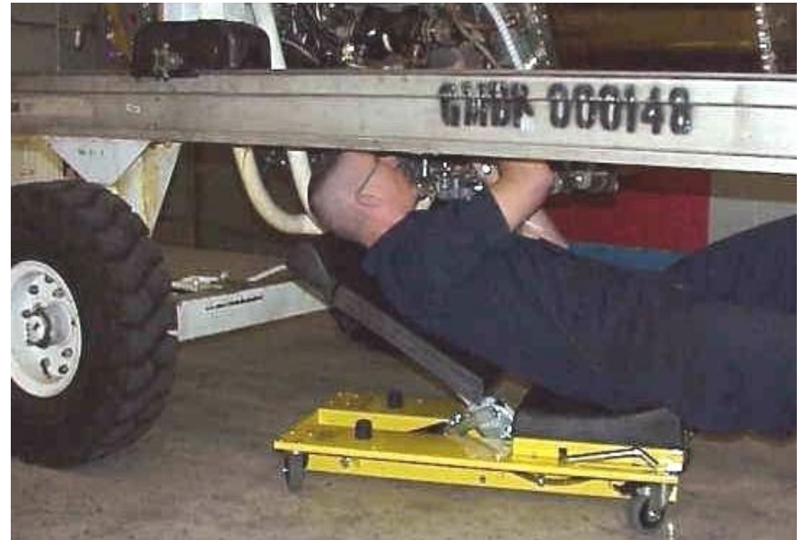
Ergonomic Improvement: Creeper supports mechanic and brings him closer to the task
