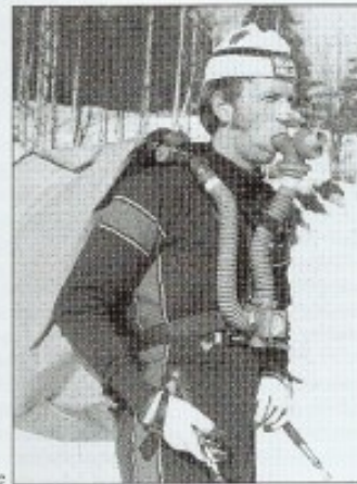
Figure 82 Application of the classic Douglas bag method for measuring aerobic energy output during different types of exercise. The skier shown in (c) carries a three-way stopcock and a stopwatch on his chest to record the time during which the expired air is collected in the Douglas bag. The stopwatch automatically starts and stops when the stopcock is turned.
