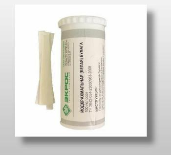
The iodine produced in the presence of starch turns the paper blue.
