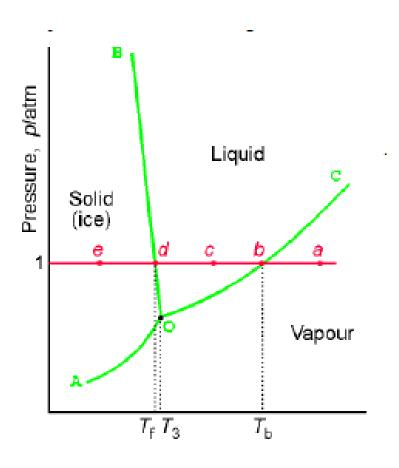
**Line OC** (liquid-vapor line) shows the boiling point of water as a function of pressure. For all the points along this line f = 1
