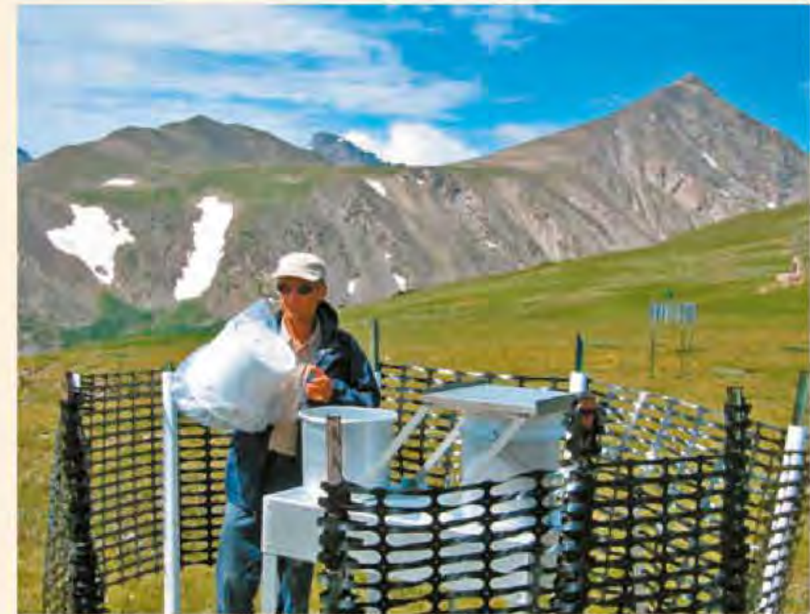
Figure A Measuring Deposition A wet deposition collector is serviced on Niwot Ridge, Colorado. The bucket on the right is covered except during precipitation events. (Courtesy of Mark Losleben.)
