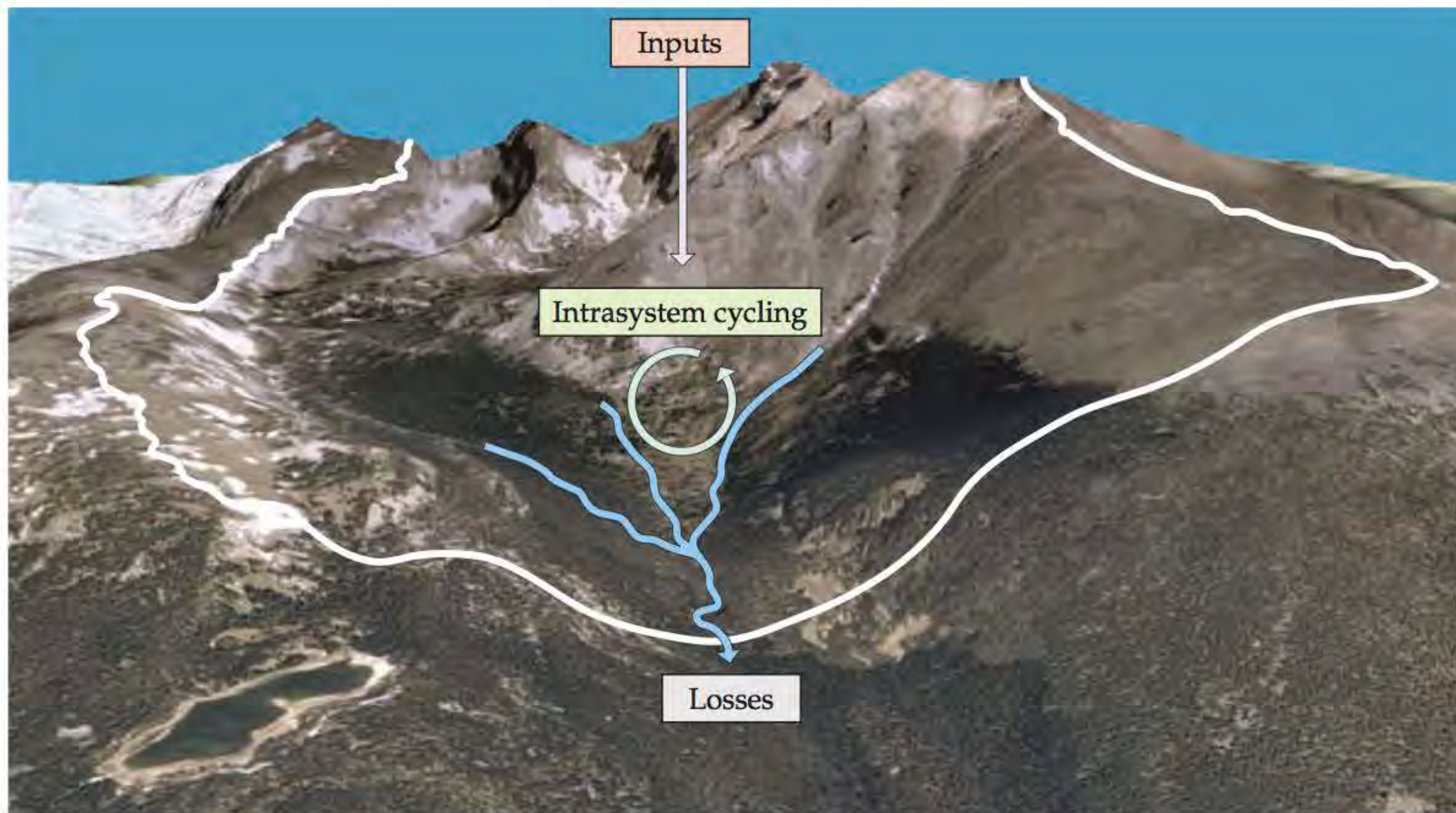
Figure 22.12 Catchments Are Common Units of Ecosystem Study A drainage basin (known as a catchment or watershed) associated with a single stream system (blue lines), with boundaries determined by topographic divides (outlined in white), is a unit commonly used in terrestrial ecosystem studies to measure inputs and outputs of nutrients. This catchment is the upper Hunters Creek basin, draining the south side of Longs Peak in Rocky Mountain National Park.
