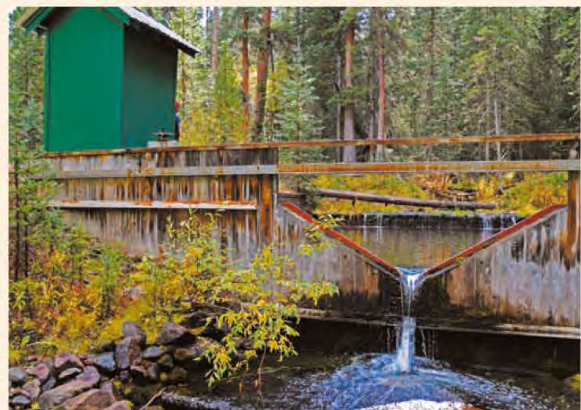
Figure B Measuring Water Flow A weir on Fool Creek in the Fraser Experimental Forest, Colorado.
