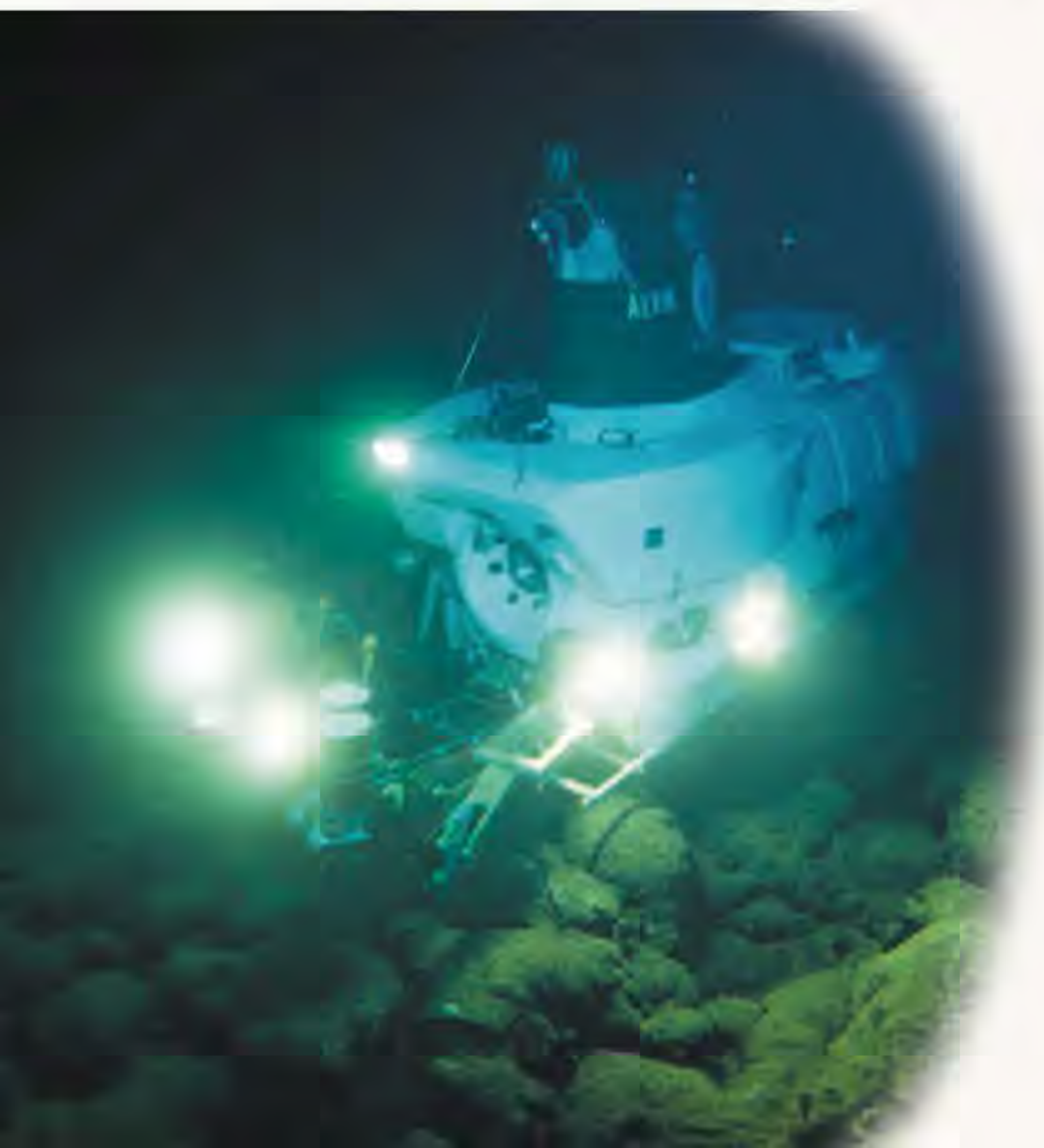
Figure 20.1 Alvin in Action The deep-sea submersible craft Alvin was instrumental in locating and exploring the first known hydrothermal vent site in 1977. The Alvin can carry two scientists and is equipped with video cameras and robotic arms for collecting specimens from the seafloor.
