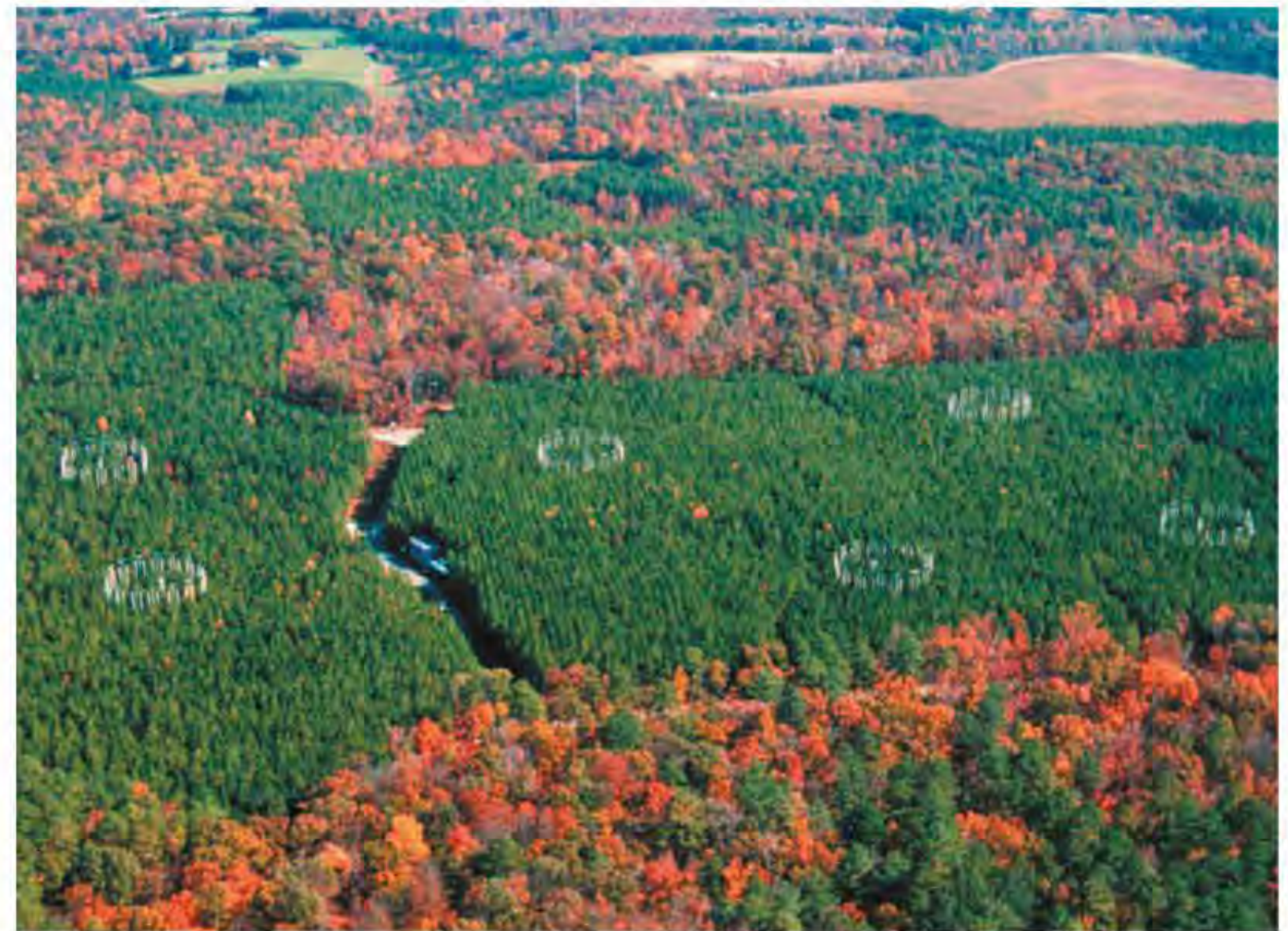
Figure 25.4 A FACE Experiment The circles visible in this aerial photo are free-air CO 2 enrichment (FACE) treatment rings in a loblolly pine ( Pinus taeda ) forest in the Duke Forest in North Carolina. Carbon dioxide is released from plastic pipes surrounding treatment plots at a rate calculated to raise the CO 2 concentration to 200 ppm above ambient atmospheric CO 2 concentrations. (Courtesy of Evan DeLucia.)
